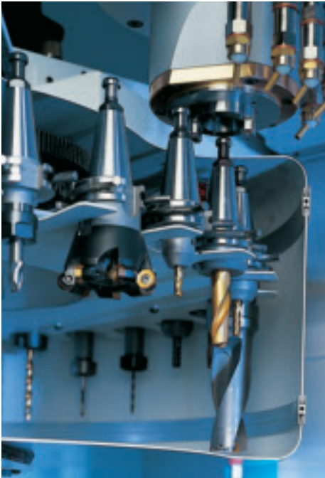
The compact pick-up changer comfortably fits 24 tools.
