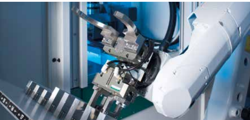
Handling of blanks as well as pallets with 6 axis articulated-arm robot
