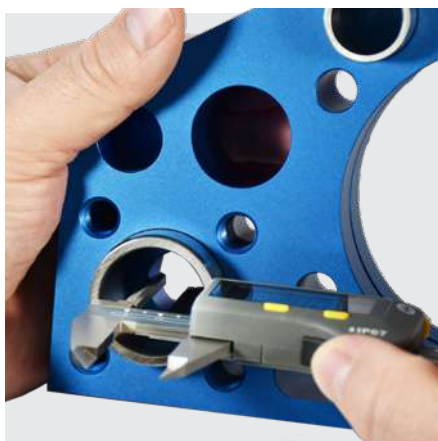
Deep measurement with S_Cal EVO Smart DM
