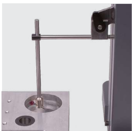
Internal groove measurement with accessories 930-2108, 930-2110 and 905-2207
