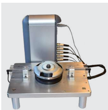
Capacitive probes connected to a D200S.
