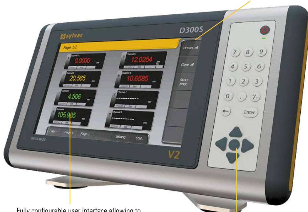
Fully configurable user interface allowing to define the number of displayed channels per screen
