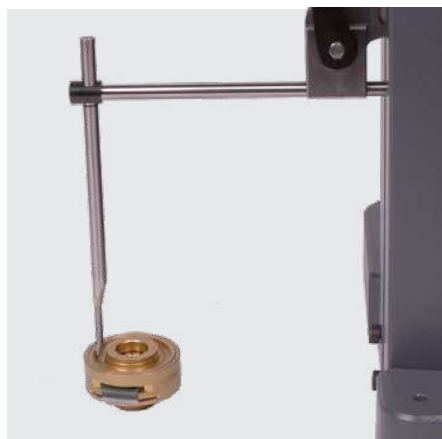
Depth measurement with accessories 930-2108 and 930-2105
