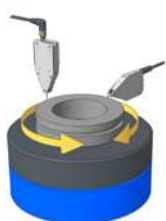
Circular geometry measurement on rotary table
