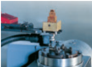
Gripper ITS 50 (50x50mm)
