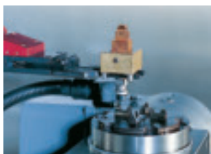
Gripper ITS 50 (50 x 50 mm)
