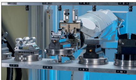
Articulated-arm robot: handling of pallets and blanks with a single system
